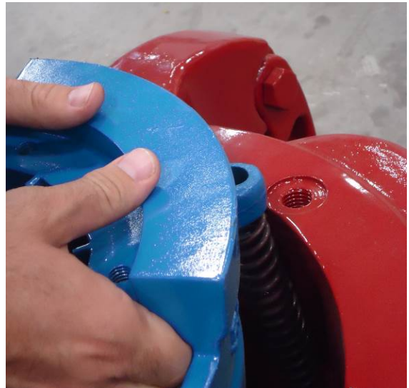
Figure 3 – Compressing spring to install slip
