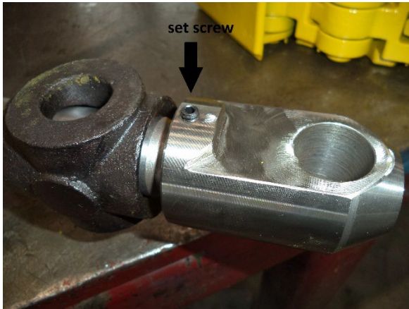
Figure 3: Set screw loosened
