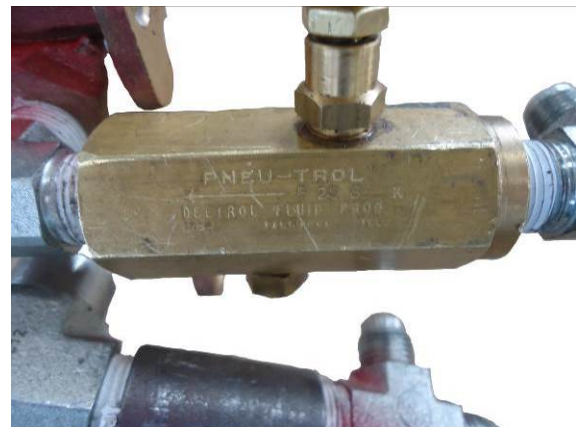
Figure 17: Valve (p/n 060061) points toward treadle
