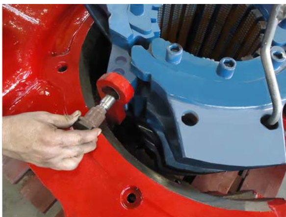
Figure 10: Slip Change – removing retainer pin
