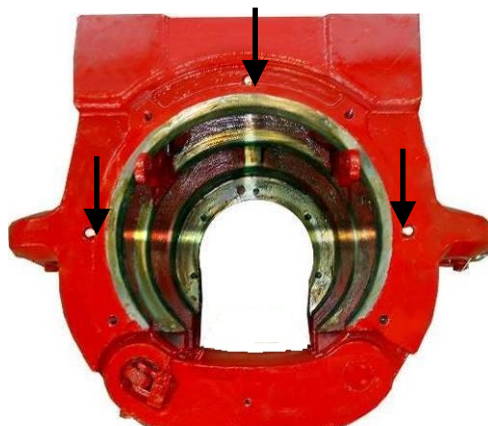
Fill grease dispensers to lubricate the inside bore. The lighted areas indicate slip contact
