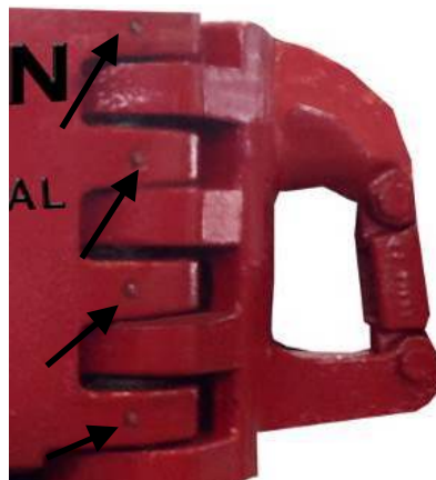
Hinge pin: grease fittings & ear contact surface (350 ton shown)
