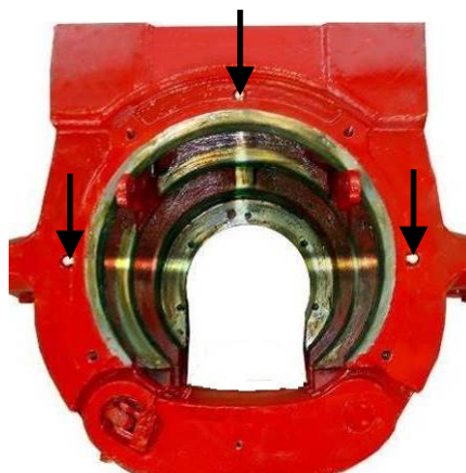
Fill grease dispensers to lubricate the inside bore. The lighted areas indicate slip contact
