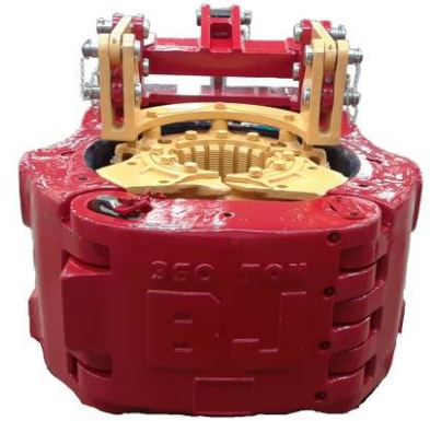
Figure 1: Snubber – shown ready for inversion
