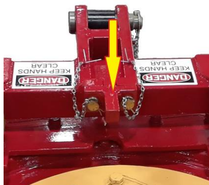
Figure 7: Bump stop installed
